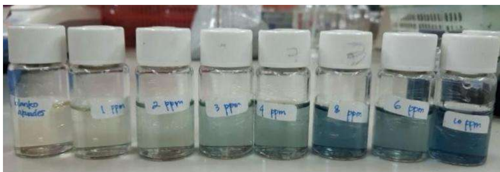
Figure 1. Standard \text{KH}_2\text{PO}_4 solution for quantitative phosphate solubilization measurement
