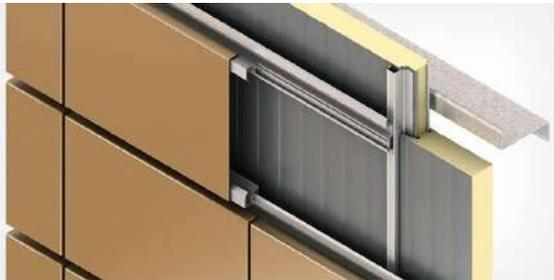
Gambar 12. Aluminium Composite Panel
